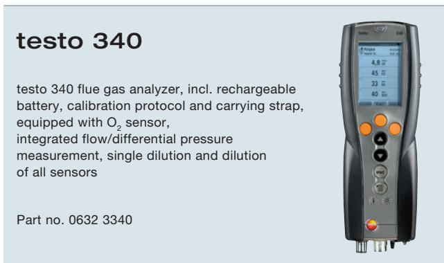
testo 340 must be equipped with a second gas sensor otherwise the analyzer cannot function. Max. 3 additional sensors can be fitted.
