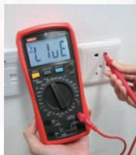
Live and nature wires identification
