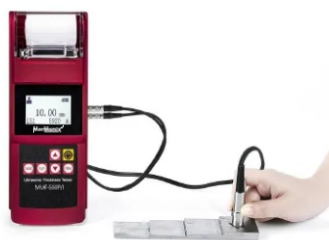
Measuring 10mm standard block
