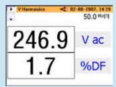
Harmonics measurements—view key harmonic factors such as distortion factor and total harmonic distortion, as well as individual harmonics up to the 30<sup>th</sup> harmonic.
