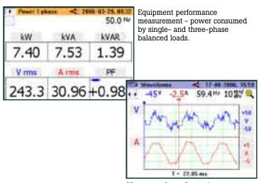
View waveforms for equipment checking and setup.
