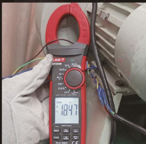
Inrush current capture (UT206B/207B/208B)
